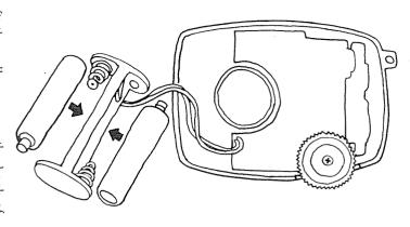
To fit the cells, remove the back of the case by prising it off gently at the bottom using a coin or small screwdriver in the slot provided. Then insert the cells in the small plastic battery holder, with the flat
