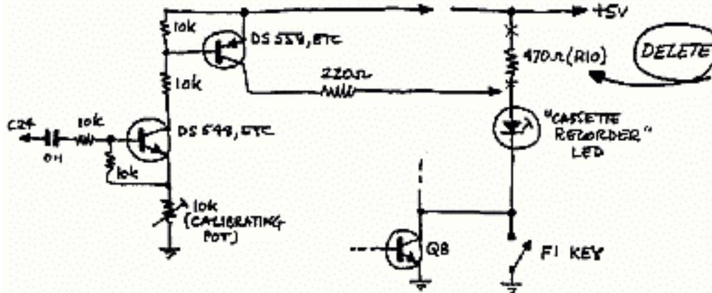
As you can see, the additional circuitry required is quite simple and involves only two low-cost transistors, four resistors, a capacitor and a preset pot for calibration. Basically, the circuit detects the positive peaks of the replay signal and amplifies them to modulate the current drawn by the LED. The 10k pot may be set so that full LED brightness is achieved only when the positive peaks of the replay reach an amplitude sufficient to ensure reliable loading.
