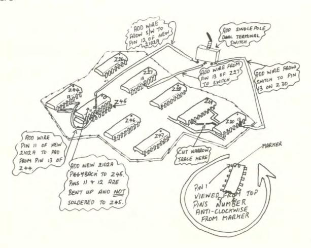
Those who haven't worked with i.c's before will need to know how the pins are numbered. With the pins downward, one end of the case is coded. Usually the marking is a tiny hole over one corner - the nearest pin is number 1. If this hole is missing, one end will have a semicircular recess. The first pin, moving anti-clockwise from the recess, is Pin 1.
